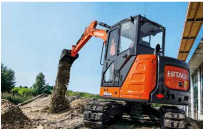
The short-tail swing radius makes the ZX65USB-6 ideal for working in tight spaces.
