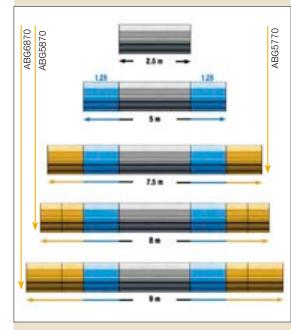
Max. paving widths with VB 88 screed
