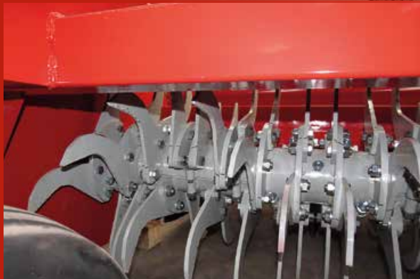
Miller's segmented shaft
