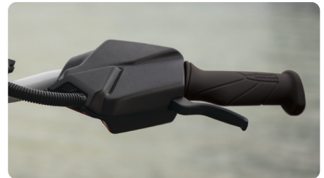
iBR® – Intelligent Brake & Reverse Exclusive to Sea-Doo®, iBR stops the watercraft sooner and provides more control and maneuverability at low speeds and in reverse.
